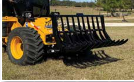
Brush Grapple (moving debris off roads)
