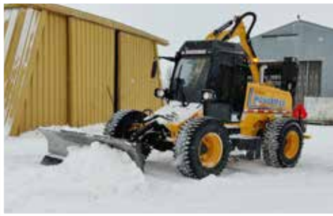
120in Snow Plow with Hydraulic Angling
